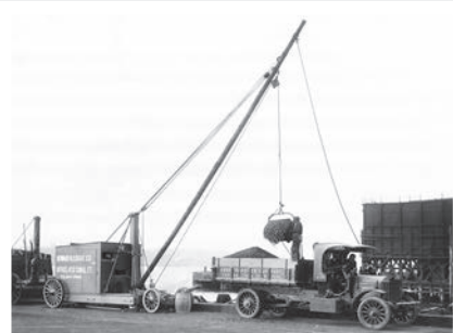
May Photo: One of F. C. Austin's various ventures after selling his original line to Western Wheeled Scraper produced excavators. This 1919 No. 5 Skimmer is equipped with a four-cylinder, 6 x 7½ gas engine and, according to the blurb accompanying the image, the "latest type of rear-dump bucket!" (F. C. Austin Company, Inc. - Austin Machinery Corporation image, Harry E. Young II Papers, HCEA Archives)
